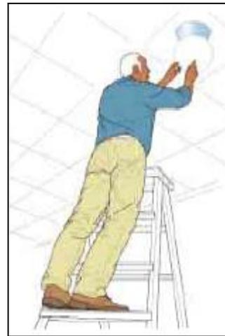
5. AVOID SIDE ON WORKING WHERE POSSIBLE-THIS IS LESS STABLE, TRY TO POSITION THE STEP LADDER HEAD ON TO THE WORK TASK AREA
